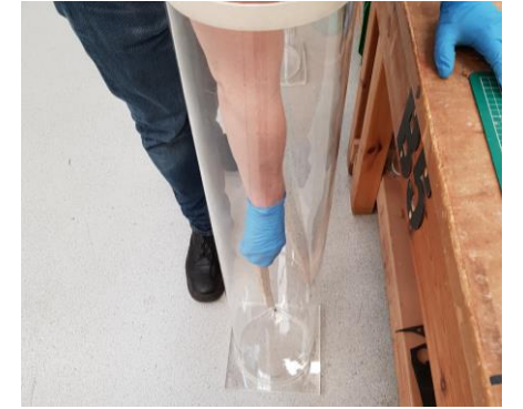
4 – Assembly of the base to the tank walls.
