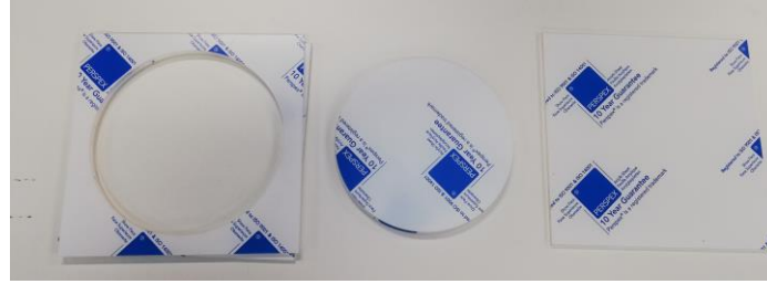
2 – The Bases are cut from 6mm acrylic.
