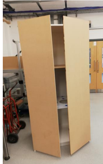
6 – Assembled PBR housing
