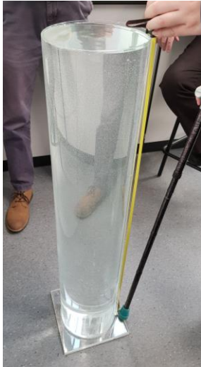
5 – IP68 submersion test for suitability around lighting system.
