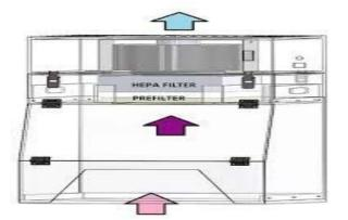
Recirculating fume hoods must not be used for highly toxic chemicals, or for regular use of toxic and/or flammable solvents in large quantities. They are not suitable for:
