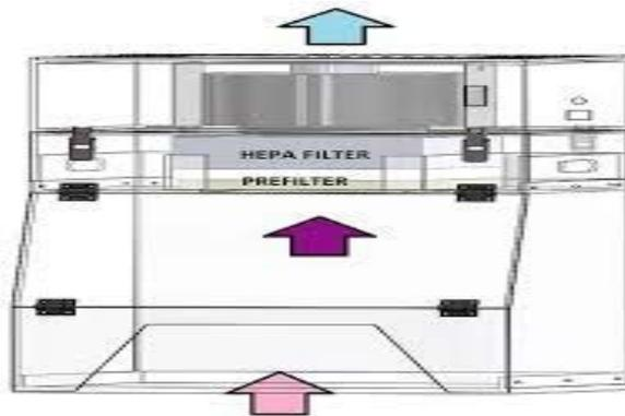
Recirculating fume hoods must not be used for highly toxic chemicals, or for regular use of toxic and/or flammable solvents in large quantities. They are not suitable for:
