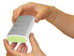
Fig. 7 Upon receiving the signal, the LED light bulb of the corresponding container is turned on.
