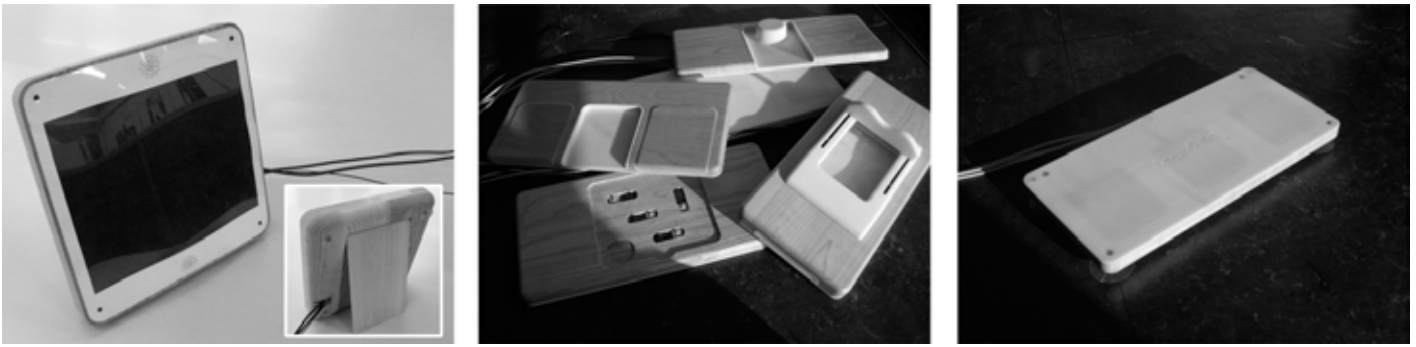
Fig. 4. Click-It contains an output module (left), four input modules (middle), and a base module (right).
