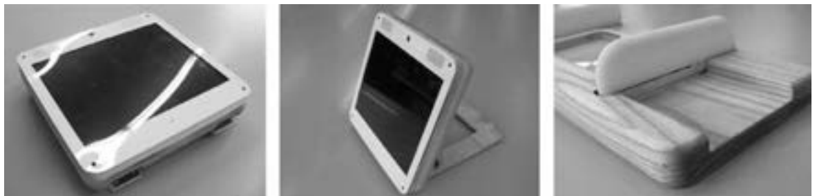
Fig. 9. The output module can be used horizontally (left), and tilted (middle). The booklets can be easily placed in a track (right)
