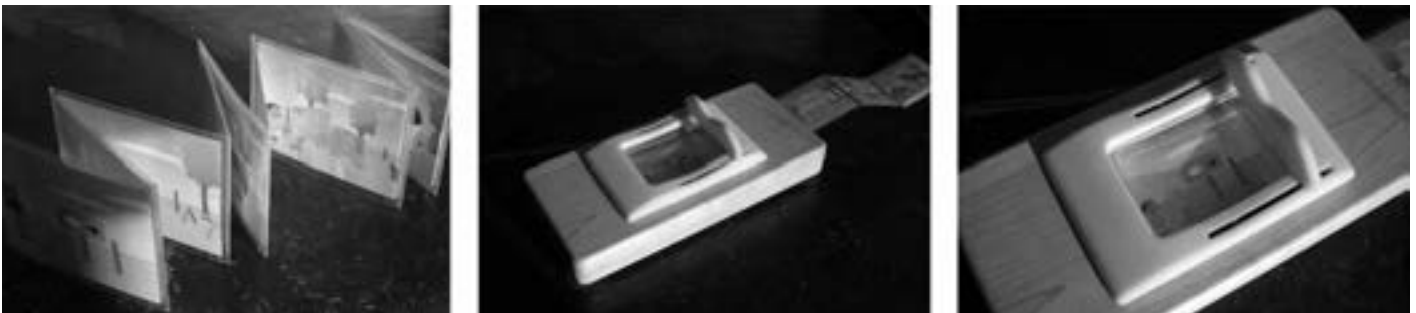
Fig. 5. The linear story booklet (left) can be inserted in the story-reading module (middle); the scene behind the viewer (right) is animated on the output module.
