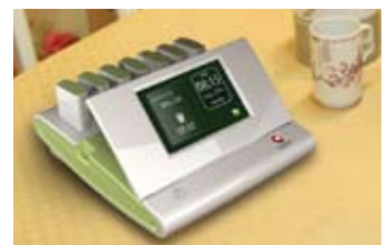
Fig. 5 The touchscreen panel with adjustable angles (0°~45°)
