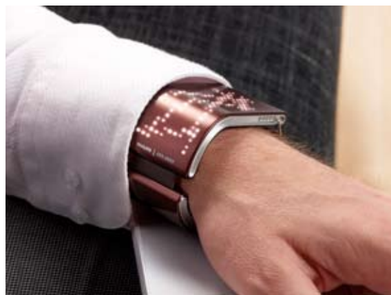
Figure 2. The EmoBracelet is an integrated emotion sensing and rendering device worn on the wrist.
