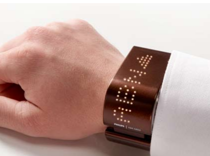
Figure 8. EmoBracelet in information mode, acting as a tickertape display with stock info.
