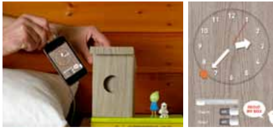
Fig. 3 The Birdbox alarm clock; the product consist of a simple box and a mobile phone application.
