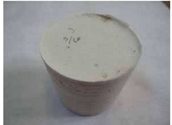
Fig. 1. Articles are cast in separate plaster cylinders
