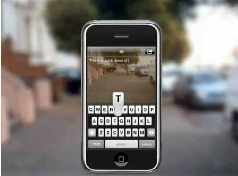
Figure 2: "Type n Walk" screenshot of iPhone application demo video by 'Type n Walk,' which augments a live video feed from the built in camera in the background of the typing area. This allows to pay undivided attention to the screen and watching the immediate path ahead at the same time.
