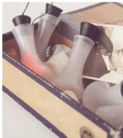
Fig. 2 "Message in the Bottle", an answer phone consisting of glass bottles which capture messages. The product can be experienced through its materiality; users may collect the bottles that contain special messages. In this concept, the non-materiality of voice messages is captured in a tangible object.
