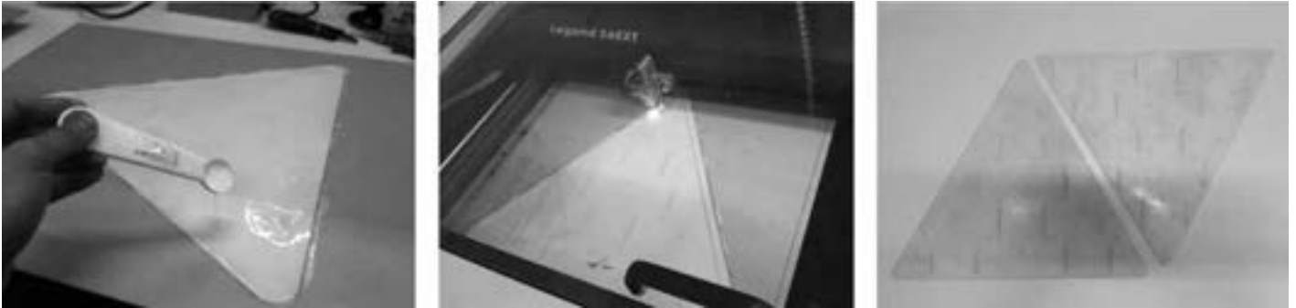
Fig. 2. Silicone rubber in the mould (left). Laser cutting the openings of 'eye' apertures with embedded SMA wires (middle). RModular silicone skin (right).
