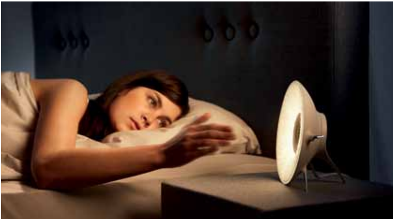
Fig. 4. Lazy snooze. In the morning, waving in front of the Wake-up Light suffices to activate snooze.
