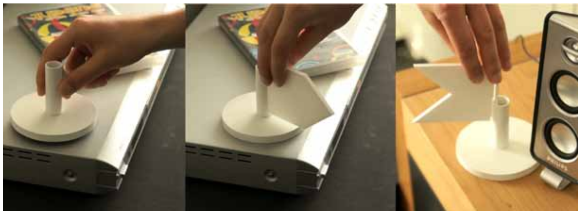
Fig. 3. Placing a Node on a device (left), placing a network start point on a Node (middle) and placing a network end point on a Node (right).
