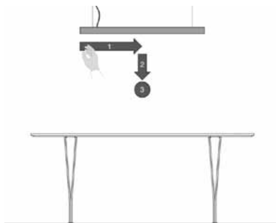
Fig. 2. Diagram showing the dining room table fixture suspended above a table. The original initiation gesture required users to: (1) move their hand horizontally from the side to just below the middle of the lamp, (2) move it vertically downwards, (3) hold it still for two seconds.
