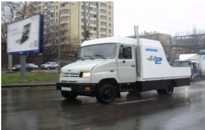
Hybrid cargo city car with ICE using hydrogen produced from methanol in a thermocatalytic converter
