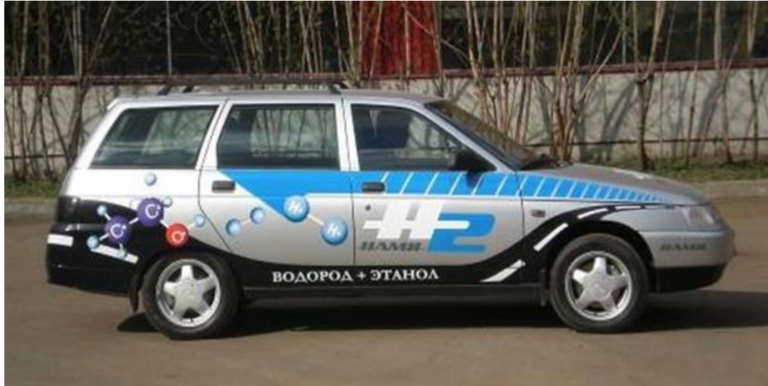
Car VAZ-2111 using hydrogen - ethanol mixtures with the production of hydrogen on board
