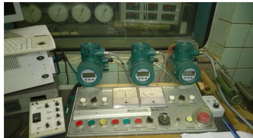
Motor bench control desk with DME and NG flow meters
