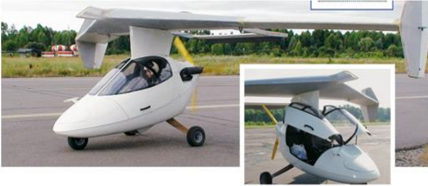
KAI-81 Superlight aircraft with Pivoting wing Patent (RU) N2277496
