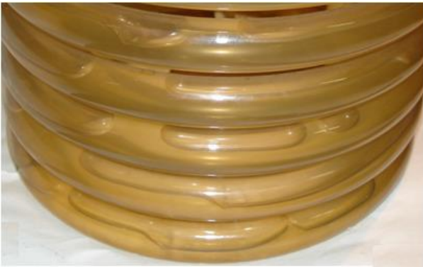
Slug flow in coil tube
