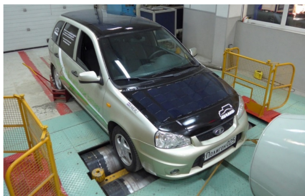
Experimental electric vehicle with photovoltaic auxiliary energy system (2017-2018)
