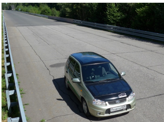
Experimental electric vehicle with photovoltaic auxiliary energy system (2017-2018)
