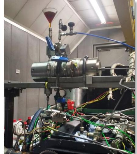
Testing of waste coffee ground derived biodiesel
