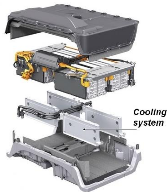
High-voltage car battery Audi A3 e-tron PHEV-20 with four cooling plates which regulate the temperature of the eight modules
