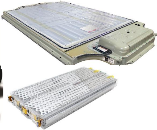
High-voltage car battery Tesla Model S consists of 16 battery modules with liquid cooling system
