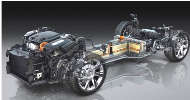
T-shaped lithium-ion high-voltage car battery Chevrolet Volt with aluminum cooling plate
