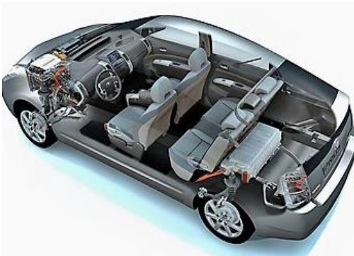
High-voltage car battery Toyota Prius with air cooling
