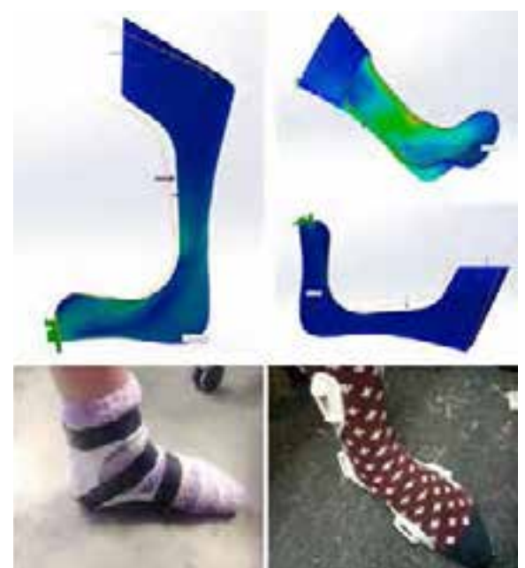
Figure 3. Early printed orthosis and strength analysis
