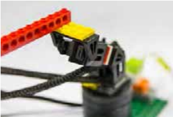
Fig. 1. Depicted above are the created actuators, two pivoting and one rotational actuator. In the left picture a square white brick is visible, this is a light sensor module in the kit.
