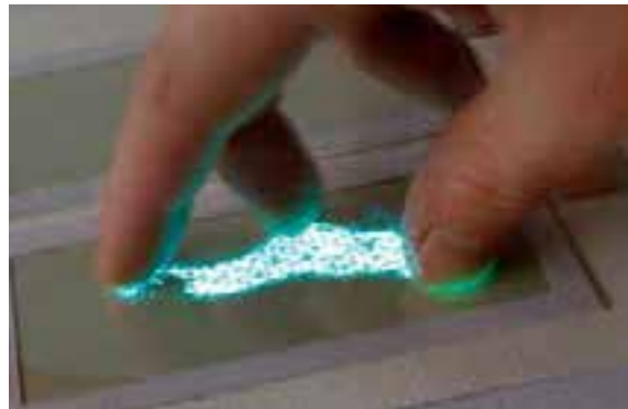
Fig. 12. Touch responsive, sounding EL surface.
