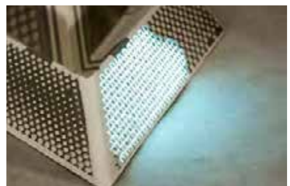
Fig. 4. EL printed on paper with perforated silver ink.
