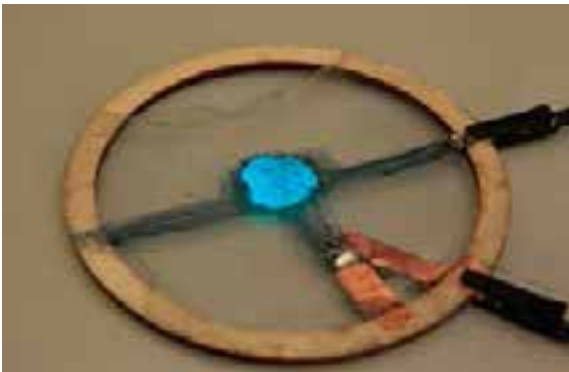
Fig. 11. EL surface hand-painted on to a dielectric elastomer.
