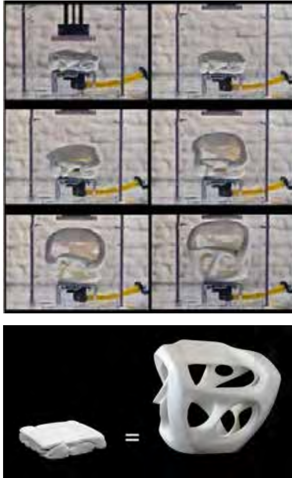
Fig. 3. Series of photographs showing how a compressed slab of shape memory foam recovers its original shape and becomes an armchair upon heating at 70°C. Shape memory polyurethane has the ability to grow up to 20 times and form soft but rigid furniture. Courtesy Carl de Smet.
