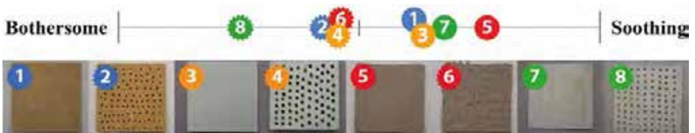
Fig. 6. The average results of 16 participants' ratings on 10 synonyms of 'bothersome' of each artifact created in the first iteration of the 'bothersome phone covers' case. Materials: wood (1 and 2), foam (3 and 4), fabric (5 and 6) and polypropylene plastic (7 and 8).
